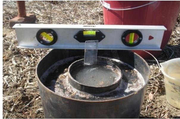
Figure 5. Installation of the double-ring infiltrometer.
